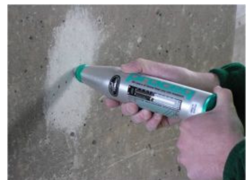
Rebound Hammer Test
